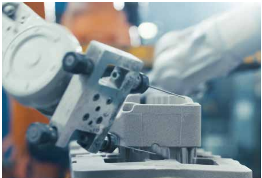
Production of inorganic cores using Inotec technology at ASK Chemicals
