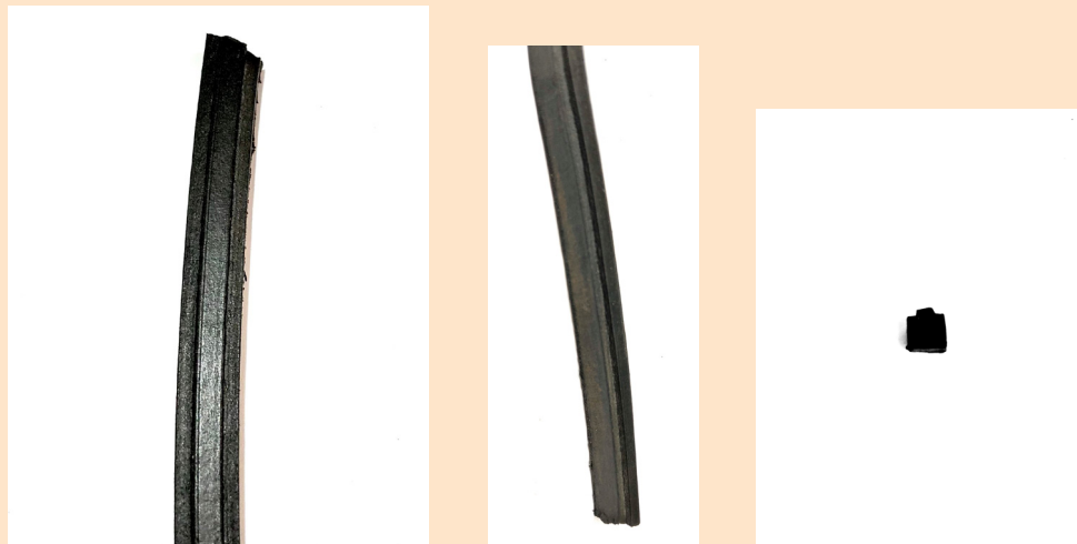
Fig. 14: Seals for the PUCB Process.
