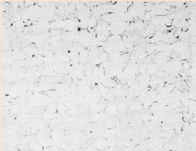
Fig. 7b: Late inoculation with inoculant containing barium
