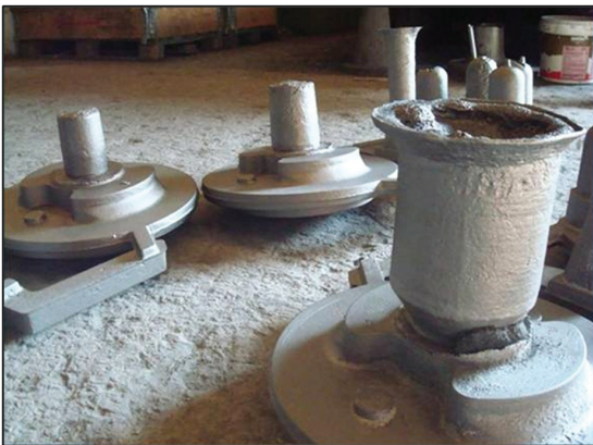
Fig.13 Yield optimisation example (stainless steel)
