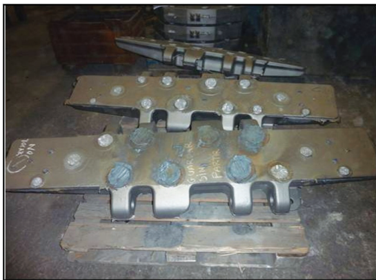
Fig.14 Yield has been improved from 58% (top) to 76% (bottom), in addition to optimising finishing times (carbon steel)
