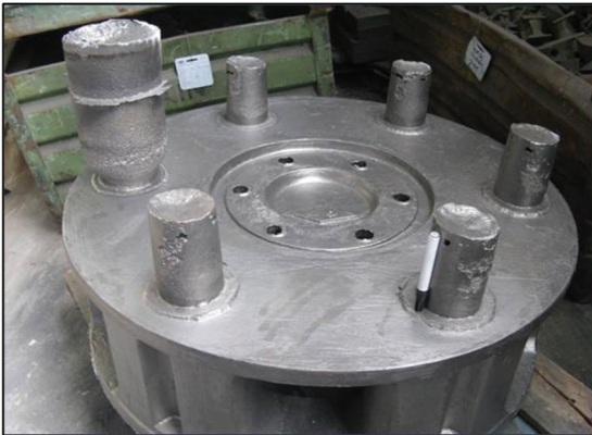
Fig.11. Manganese steel part: conventional riser (far left) versus mini-riser behaviour (middle and right)
