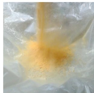
Fig 1: Powder resin without dust suppressant
