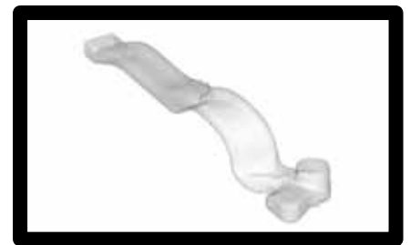
Sequence 3 Core completely gassed \leq 4 sec.
