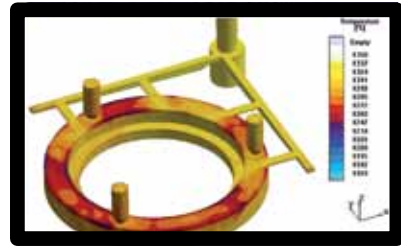
Sequence 3 Completely filled mold, very cold tempera-
