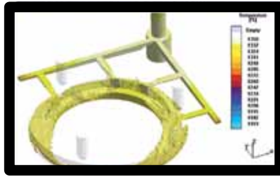
Sequence 2 Partly filled mold
