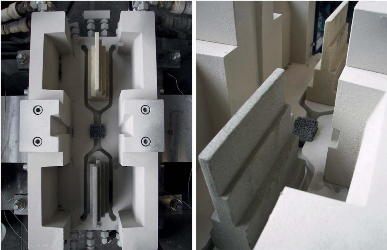
Figure 4: Test setup: Inotec core at the front, cold-box core at the back
