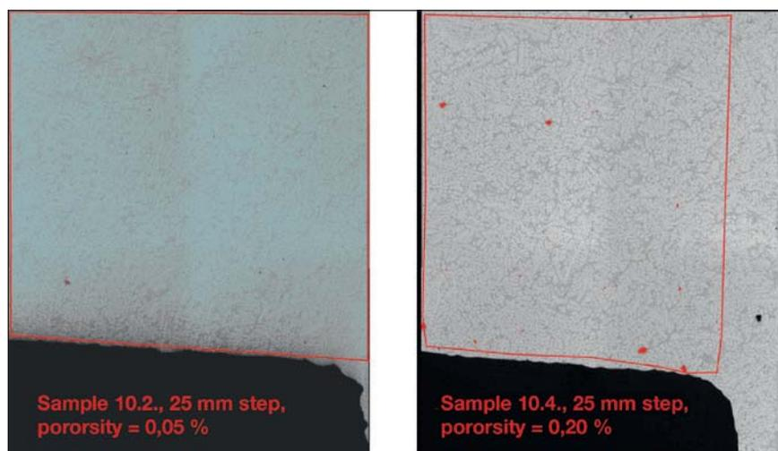
Figure 10: Porosity according to wall strength
