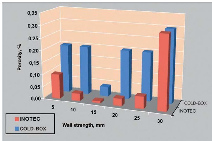
Figure 9: Porosity comparison between castings with an inserted Inotec and cold-box core
