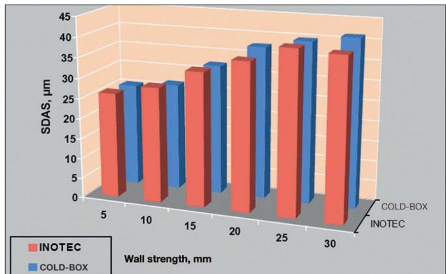
Figure 8: Secondary dendrite arm spacing (SDAS) in accordance with wall thickness
