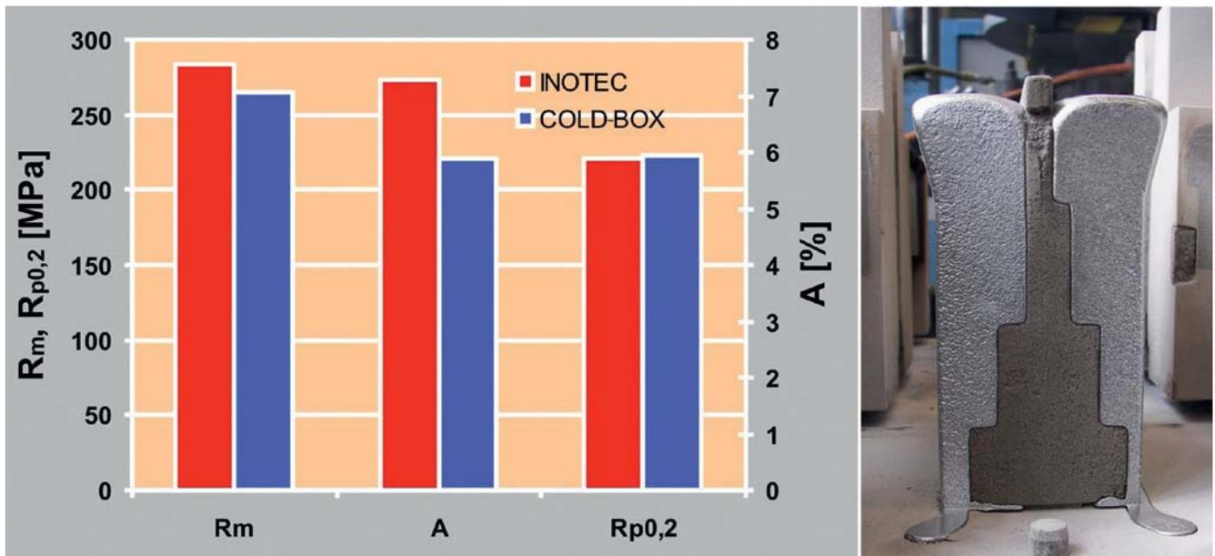
Figure 11: Results of the tensile test for cores with a free surface to air
