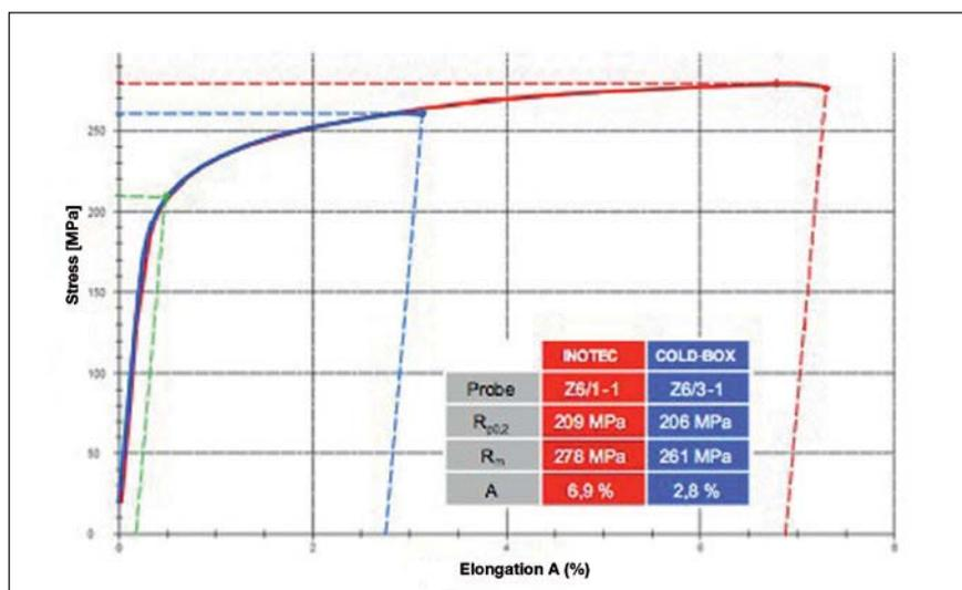
Figure 13: Comparison of the stress-strain curves between castings with an inserted Inotec and cold-box core
