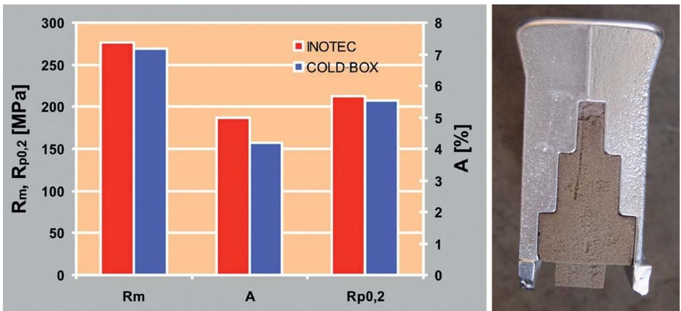
Figure 12: Results of the tensile test for fully enclosed cores
