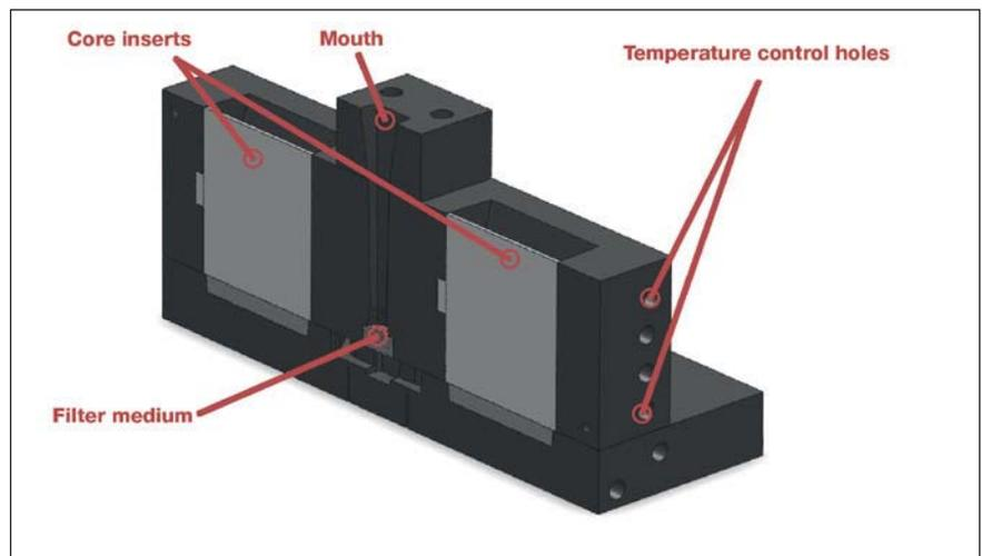
Figure 2: Full-section view of a dual-step plate die mould. Left die half with Inotec core, right die half with cold box core.
