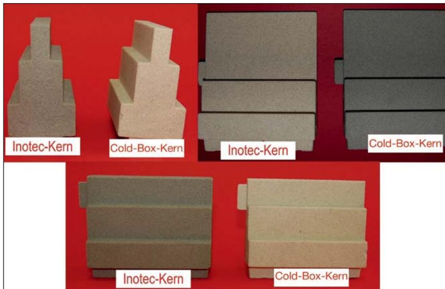
Figure 5: Core variants 1 (for fully enclosed) and 2 (for cores with a free surface to air)
