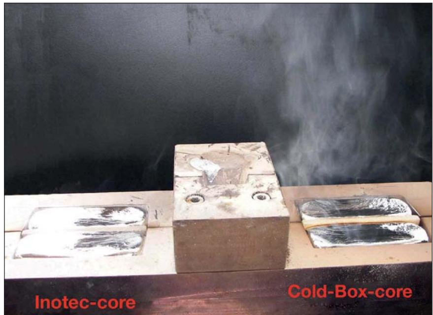
Figure 6: Strong emissions of the cold-box core (open core)
