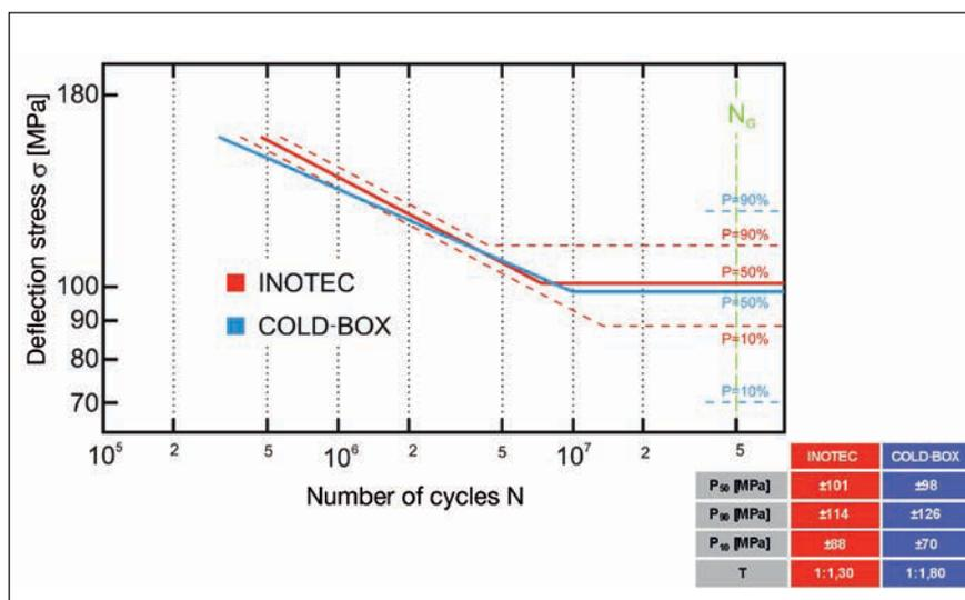
Figure 14: S-N Wöhler curves for different failure probabilities (rotational bending fatigue test)
