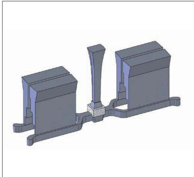
**Figure 1:** 3-plate tool with central casting and virtual casting of the stepped plates
