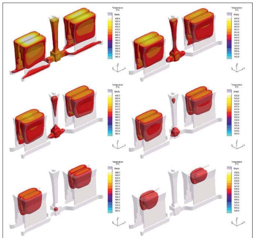
Figure 3: Solidification simulation: Comparison between Inotec core (left) and cold-box core (right)
