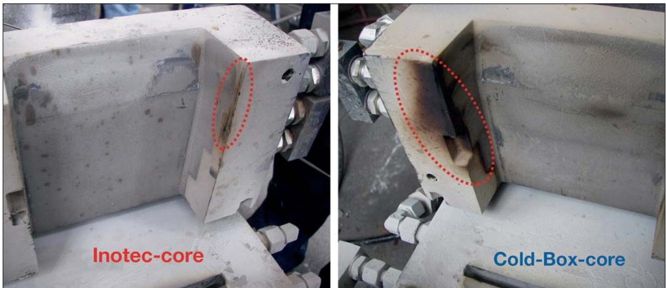
Figure 7: Resin formation due to organic condensates by using Coldbox cores
