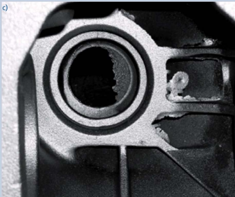
Examples of castings produced with uncoated cores: a) and b) casings for differential gears, each with 0.7 % CB per unit, 7 % additive BR 14000; c) casing for rear axle, 0.7 % CB per unit, 7 % additive BR 14000
