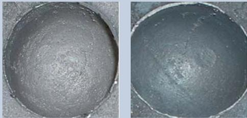
Casting test with dome core and additive BR 4048 (GJL, 1425 °C): a) uncoated, b) coated
