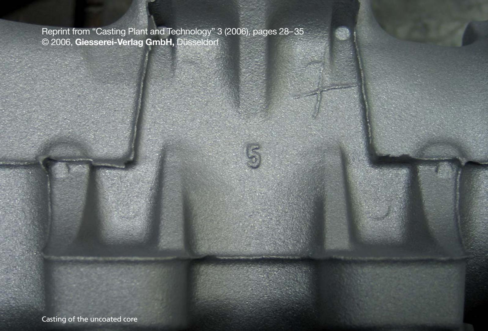
Casting of the uncoated core
