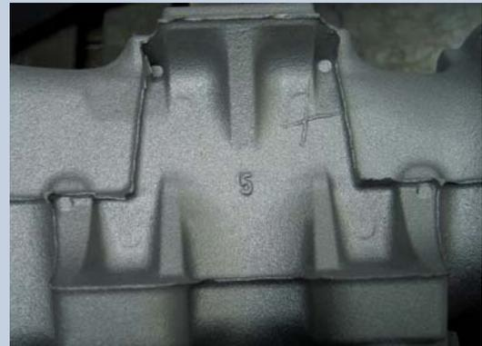
Coated – uncoated comparison: a) casting of axle inset core with (alcohol-based) coating, 0.8 % CB per unit; b) casting of the uncoated core, 0.8 % CB per unit, 2.0 % additive BR 4048
