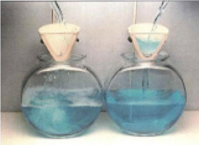
Fig. 1 Simplified laboratory demonstration of turbulence reduction through the use of reticulated ceramic filters.
