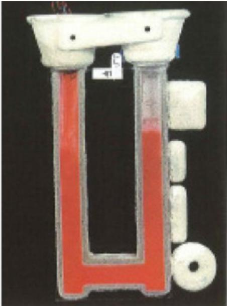
Fig. 3 Simple two vertical runner bar gating system with parts attached to one runner. A) No filter, poured down the runner without parts attached
