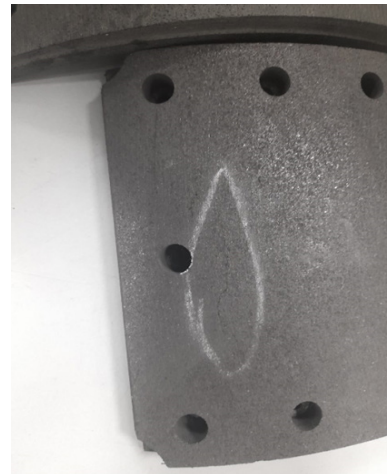
Fig 1: Truck lining with hairline crack
