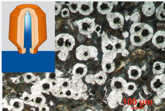
Figure 2: Reduction of graphite degradation: The fluorine-free recipe helps minimize graphite degradation in ductile iron that is usually encountered in the feeder's zone of action.
