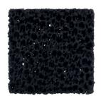
ASK Chemicals carbon bonded filters are used for ferrous alloys that may experience priming difficulties. The carbon bonded filters provide an excellent mix of priming efficiency with filtration effectiveness. A low percentage of carbon limits the possibility of contamination from carbon pick-up. UDICELL™ carbon bonded filters can be engineered in custom shapes, with a maximum dimension of 6" or 150 mm.
