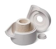
The exactfill housing system is easy to assemble within the gating and runner system. Assembly of multiple housing, at one or more levels, allows the molding and pouring of very large castings. Each piece has an outlet so you can close off either the top or bottom with the stopper. This feature eliminates the need for left or right hand versions. Also, these units are directly compatible with standard ceramic tile systems.
