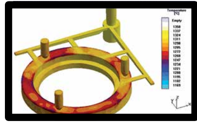
Sequence 3 Completely filled mold, very cold temperature of the cast metal after mold filling
