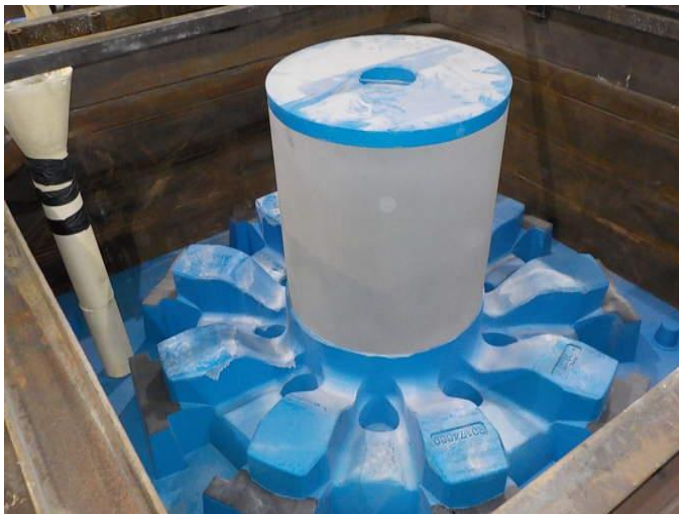
Fig. 1: The riser cap, developed by ASK Chemicals for the project, combines both insulating and exothermic characteristics. Especially size and geometry of the cast part required a tailored feeding solution.
