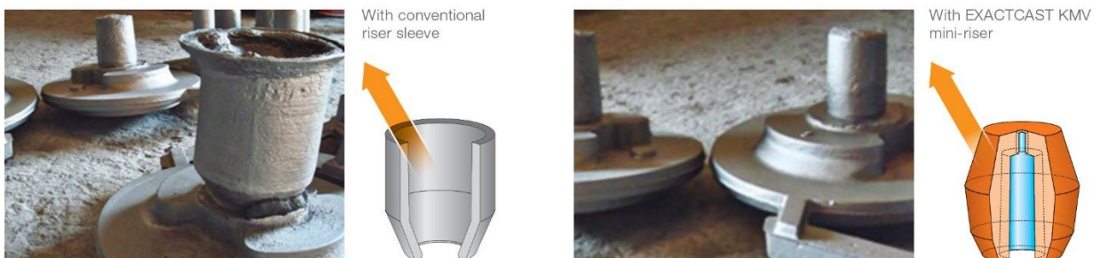
Fig. 2: The reduced riser volume and exothermic formulation (right) offer attractive saving potentials, especially in steel casting applications.
