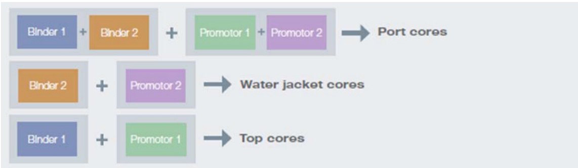
Fig.2: The modular system of the INOTEC™ technology
