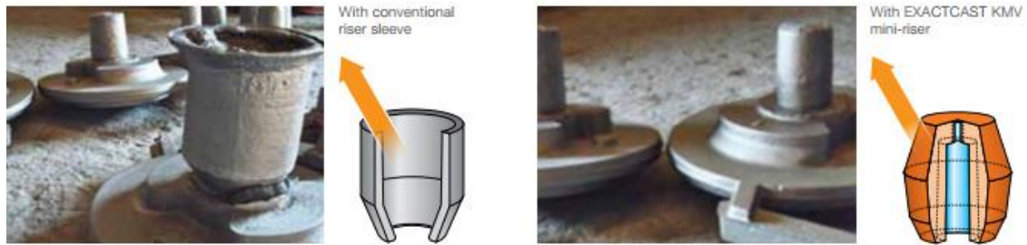
Fig. 1: The reduced riser volume and exothermic formulation (right) offer attractive saving potential, especially in steel casting applications.
