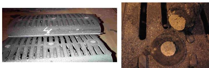
Fig. 4. The photo on the left shows a manganese steel casting fed with an EXACTCAST mini-riser, taking advantage of the reduced contact area on a particularly difficult casting geometry to feed.
