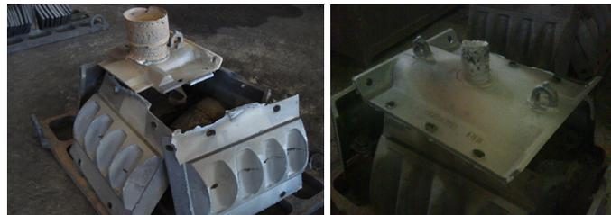
Fig. 3. The photo on the left shows a manganese steel casting fed with a standard cylindrical sleeve. The photo on the right shows the use of an EXACTCAST mini-riser on a similar casting, highlighting the significant reduction in feed metal.
