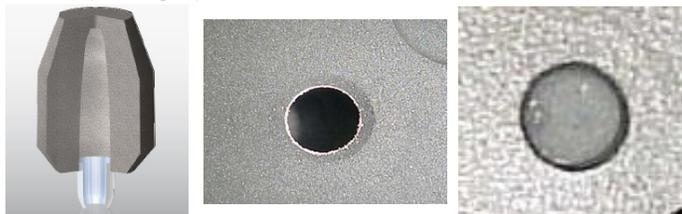
Fig. 2. The left most picture shows a cross-section of the mini-riser with metal neck breaker, followed by the finished mold with breaker contact area (middle), and lastly the casting results with the reduced riser contact area (right).
