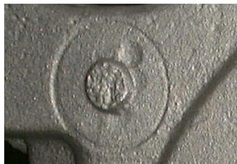
Fig.1. This photo shows the footprint of the breaker core on a casting coming from the pattern.
