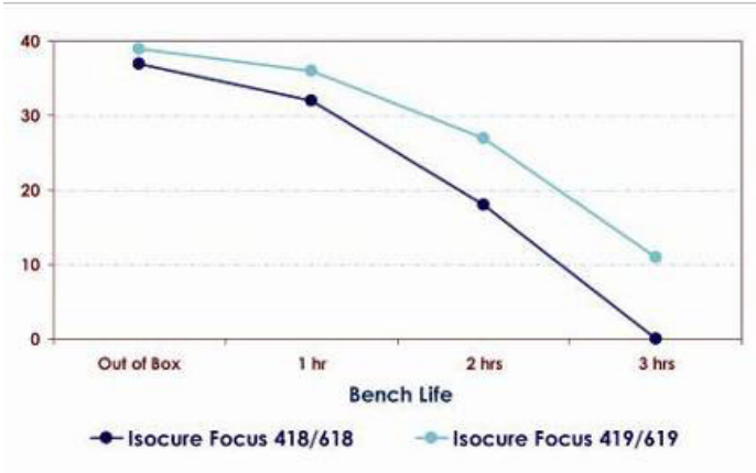
Figure 20: This graph shows the benchlife of sand and the new ESA 2011 additive for two different binder systems sand and no coating
