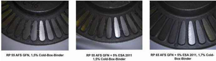
Figure 15: These brake rotor castings show the improvements with the new 2011
