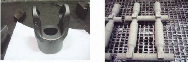
CARDAN JOINT with 70 AFS GFN sand + 5% ESA 2011 – cold box core Weight of the piece: 2.8 kg., Thickness: 35 mm., Vertical Molding Line 450mm ferrostatic pressure
