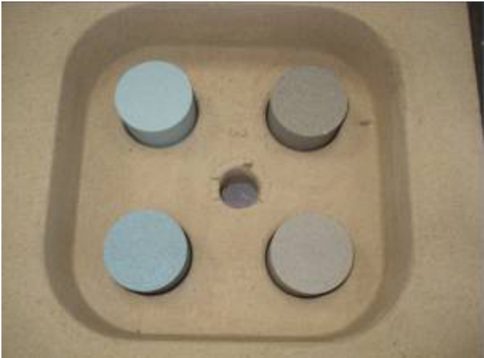
Figure 5: This is a photograph of the test casting mold and test cores for evaluating veining
