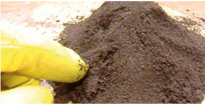
Figure 2: Testing the processability of the moulding material with a moulding material cone
