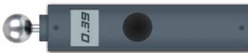
Figure 15: Moisture measuring device for determining a guide value of the mould or core residual moisture; ©Ulif Knobloch, ASK Chemicals
