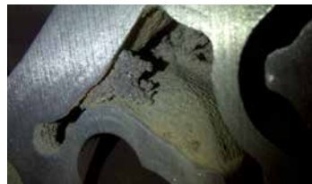
Figure 7: Penetrations in the core area caused by insufficient compaction
