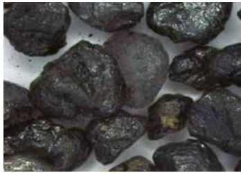
Figure 6: Mechanically well reclaimed sand
