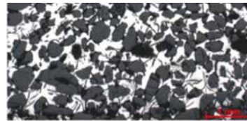
Figure 5: Left good compaction – little iron penetration, right poor compaction – strong iron penetration
