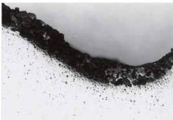
Figure 17: Penetration due to insufficient compaction 4
