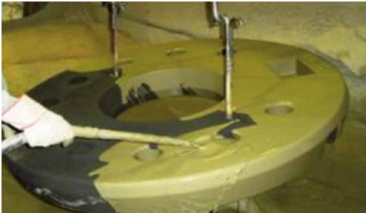
Figure 8: Flooding a core
