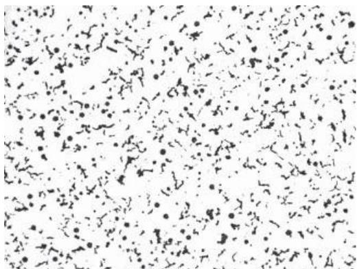
Fig. 8: CGI SiMo graphite structure from example 3, ratio 50:1, not etched
