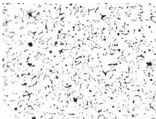
Fig. 6: CGI graphite structure from example 1, ratio 100:1, not etched
