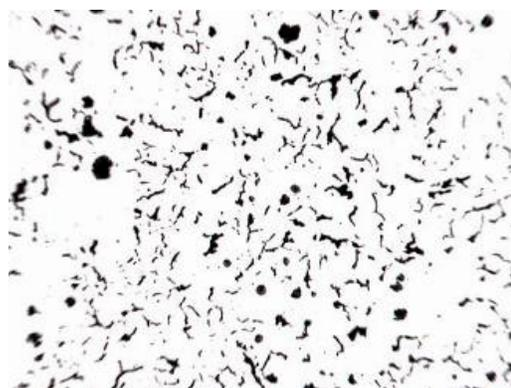
Fig. 7: CGI graphite structure from example 2, ratio 100:1, not etched
