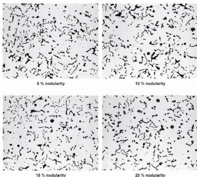
Fig. 2: CGI structure with different percentages of nodular graphite according to ISO 16211
