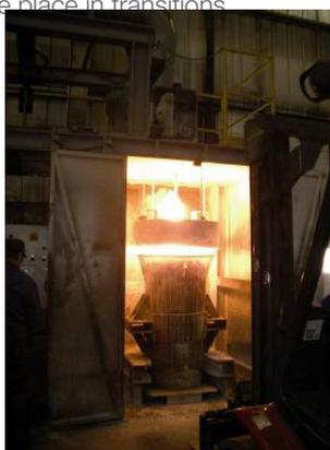
Fig. 5: Wire treatment booth for the production of CGI
