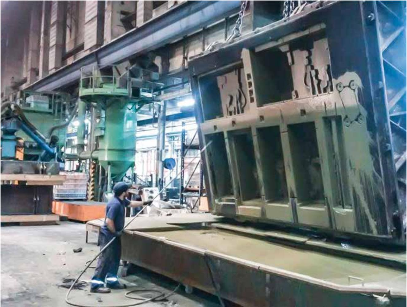
**Figure 1:** The mold is coated at the mobile flood basin.
