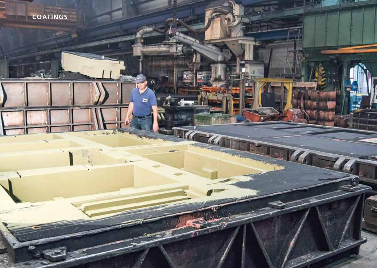
Solitec HI 703 (water-based coating) shows the user the current status of drying by means of a colour change.
