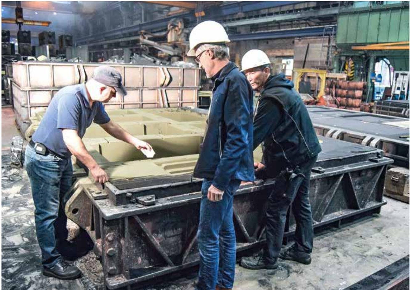
**Figure 2:** Stefan Braun, Production Manager, Ulf Schmidtgen, Segment Manager of Koenig & Bauer Gießerei GmbH, and Ulf Knobloch, ASK Chemicals GmbH (left to right), measuring the wet layer thickness.
