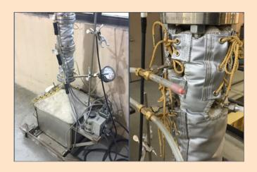
The hood stack technique is the recognized method for collecting point source emissions. The procedure calls for collecting airborne decomposition emissions from molds less than 24 hours old. The hood stack test uses Class 30 gray iron at 2,600°F as the ignition source and sampling begins immediately upon completion of metal pouring.
