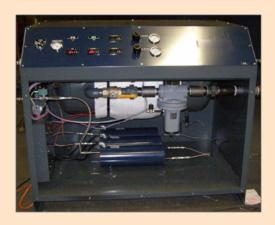
The  $SO_2$  gas is followed by a dry air purge. The purge air thoroughly distributes the  $SO_2$  throughout the tooling to ensure complete curing, then flushes residual A-E/ $SO_2$  gas from the sand. Heated purge air can be used to more efficiently distribute and carry the  $SO_2$  from the sand and out of the pattern.
