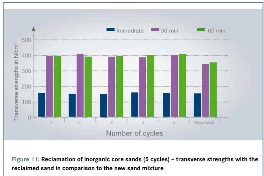
Figure 11: Reclamation of inorganic core sands (5 cycles) – transverse strengths with the reclaimed sand in comparison to the new sand mixture
