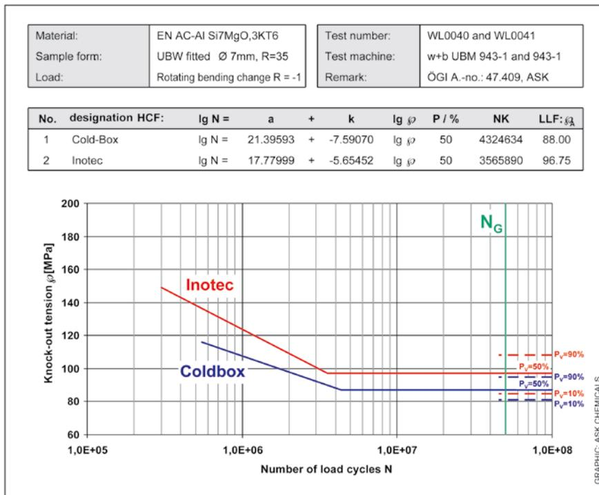
Figure 2: Rotating bending change response – Inotec (cooler base plate temperature) and Cold-Box in comparison
