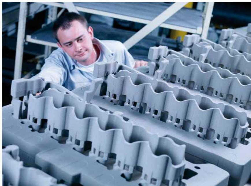
Figure 3: Core production at ASK CoreTech GmbH in Moosburg
