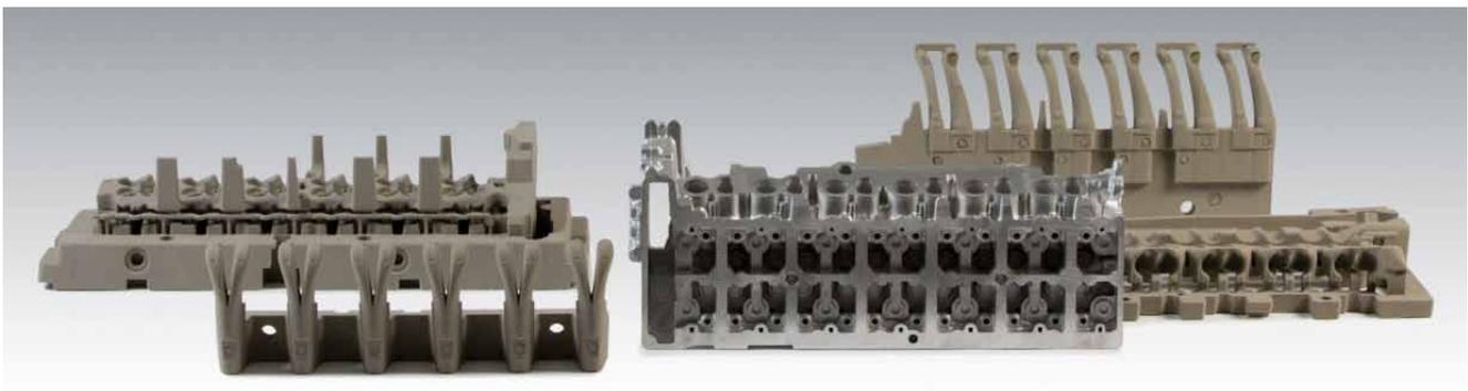
Figure 1: Cylinder head for a 6-cylinder diesel engine and sand cores.
