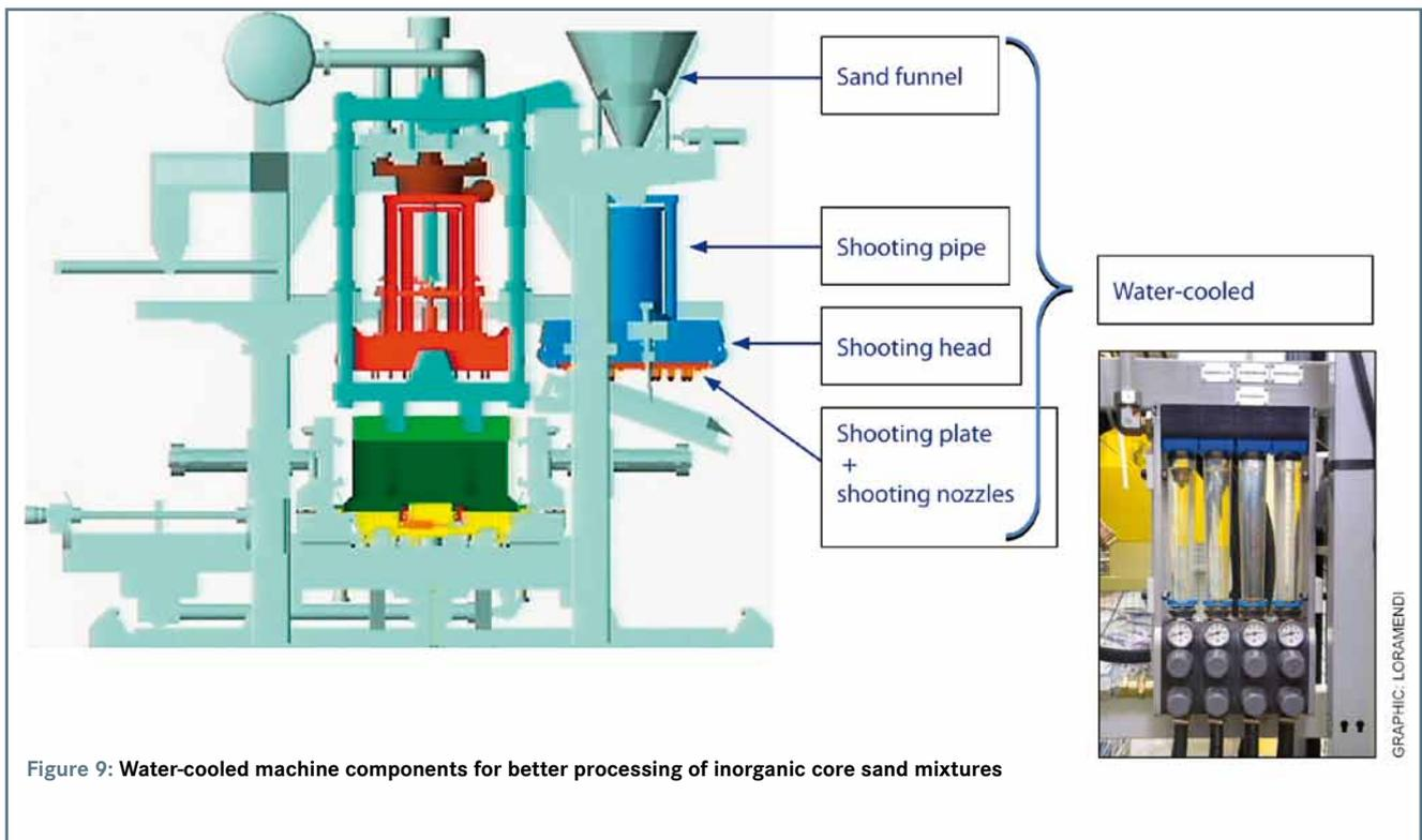
Figure 9: Water-cooled machine components for better processing of inorganic core sand mixtures
