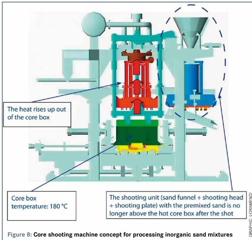
Figure 8: Core shooting machine concept for processing inorganic sand mixtures
