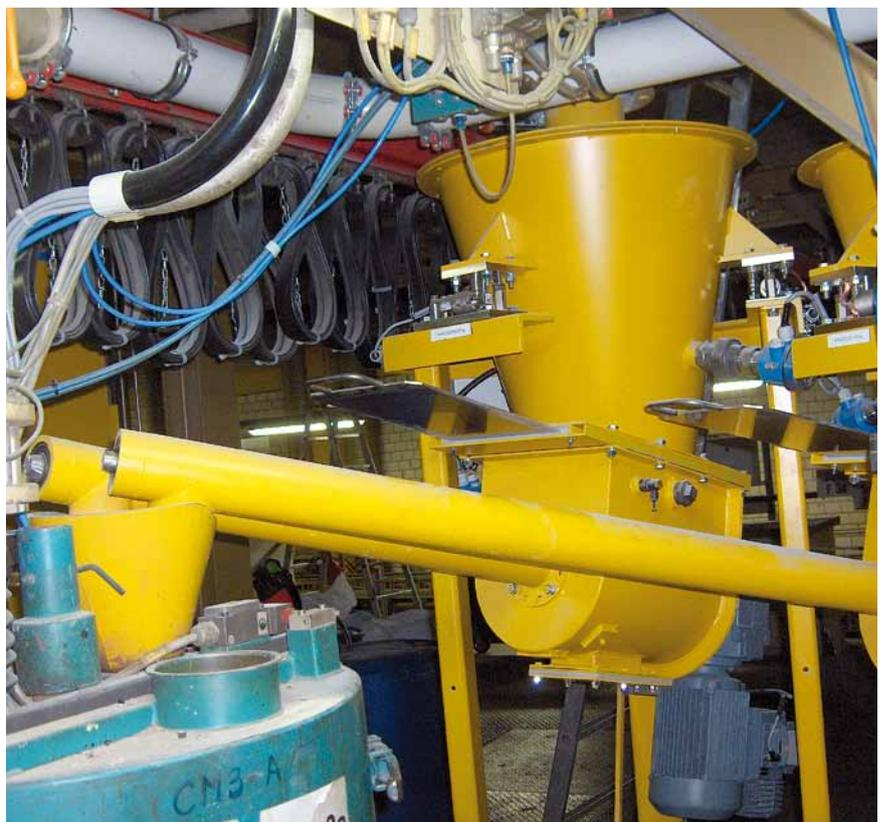
Figure 7: Screw feeder with electronic weighing cell
