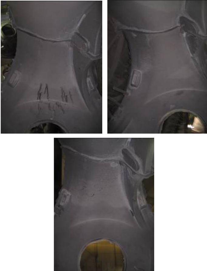
Figure 13: Clean surface after the first blasting with optimum coating application
