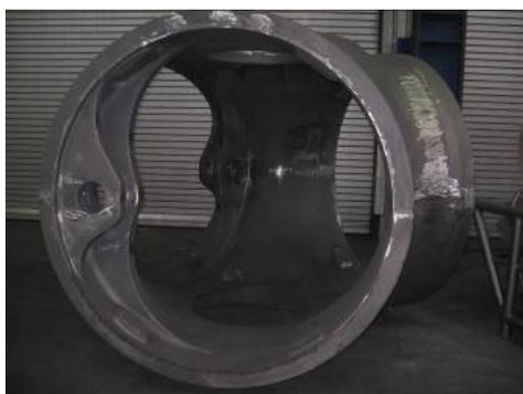
Figure 4: Rotor hub
