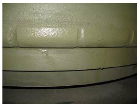
Figure 9: Sagging during spraying
