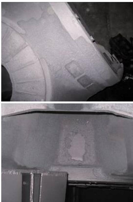
Figure 5: Casting surface of the rotor hub, casting defect – metallization
