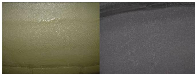
Figure 7: Sprayed core with orange skin Figure 8: Orange skin on the cast part
