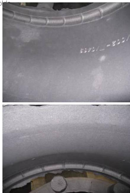
Figure 6: Casting surface following optimization of the spraying unit
