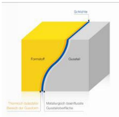
Figure 1: Application of the coating
