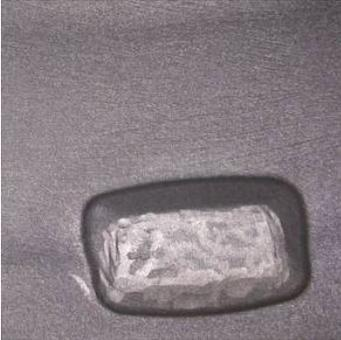
Figure 14: Flooded and repainted - casting surface with paintbrush strokes
