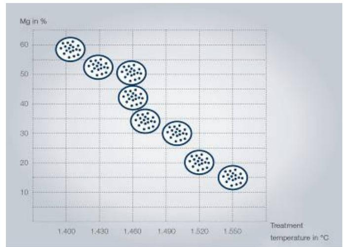
Figure 4: Mg recovery amount depending on the treatment temperature
