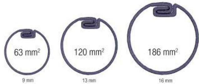
Figure 6: Cross-sectional areas of different wire diameters
