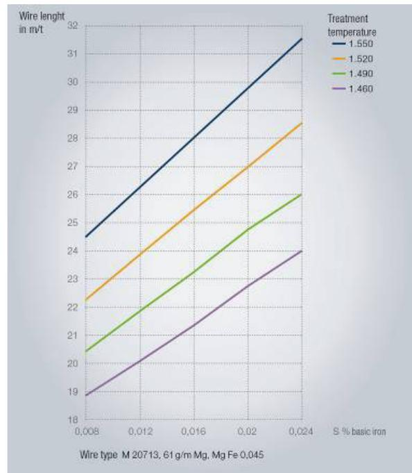
Figure 10: Wire feeding in relation to temperature and sulfur content
