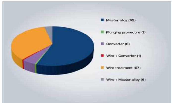
Figure 2: Breakdown of Mg treatment procedures from 165 German foundries (Nov. 2012)
