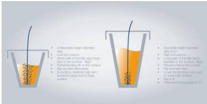
Figure 3: Influence of the ladle dimensions during the Mg cored wire procedure
