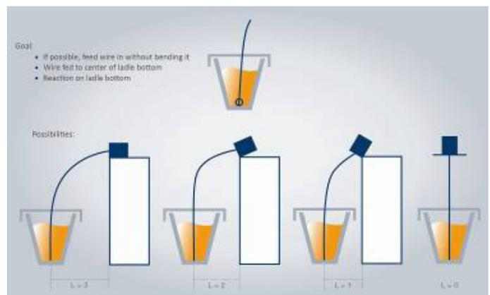
Figure 7: Methods of arranging the winding machine/treatment ladle
