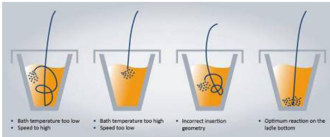
Figure 8: Behavior of the wire while being inserted into the ladle
