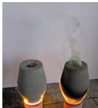
Fig. 5: Unfavorable binders in the riser can cause additional emissions to occur; left shows a waterglass-bonded riser and right shows a resin-bonded riser (ASK Chemicals Feeding Systems)
