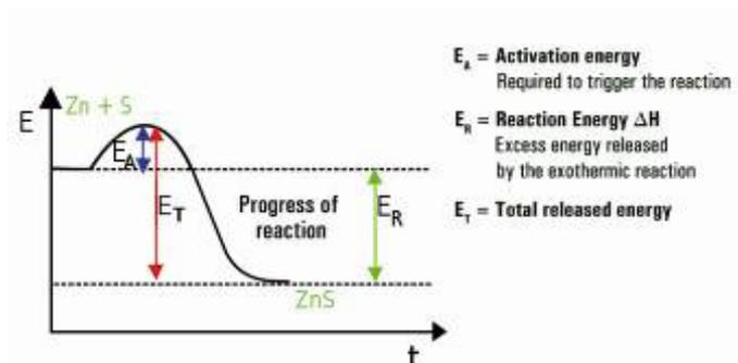
Fig. 4: Energy diagram of an exothermic reaction (source: Wikibooks.de)
