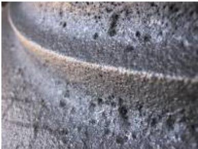
Fig. 7: Possible fluorine defects on cast pieces due to fluorine contents in exothermic riser material
