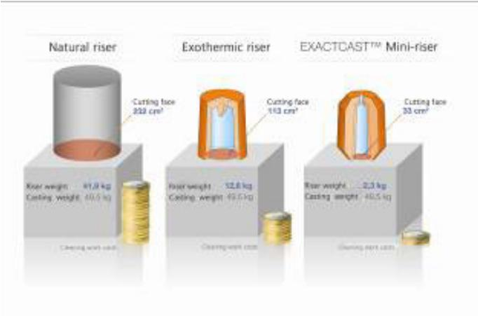
Fig. 8: Comparison of natural, exothermic and mini-risers in terms of cleaning costs (ASK Chemicals Feeding Systems)
