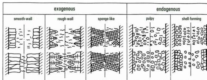
Fig. 2: Exogenous and endogenous solidification types at two consecutive times (according to Patterson and Engler, schematic)
