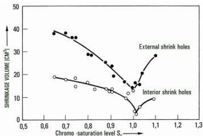
Fig. 3: Shrink hole volume of Fe-C alloys in relation to the chromo -saturation level
