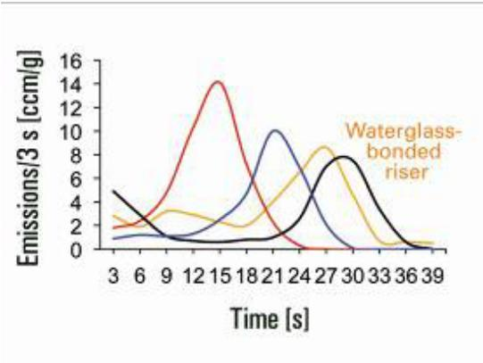
Fig. 6: Comparison of emissions of waterglass-bonded riser with various resin-bonded risers
