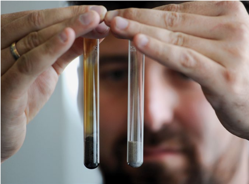
3 Combustion residues (condensate) during a lab casting test (left: conventional organic binder; right: new inorganic process)
