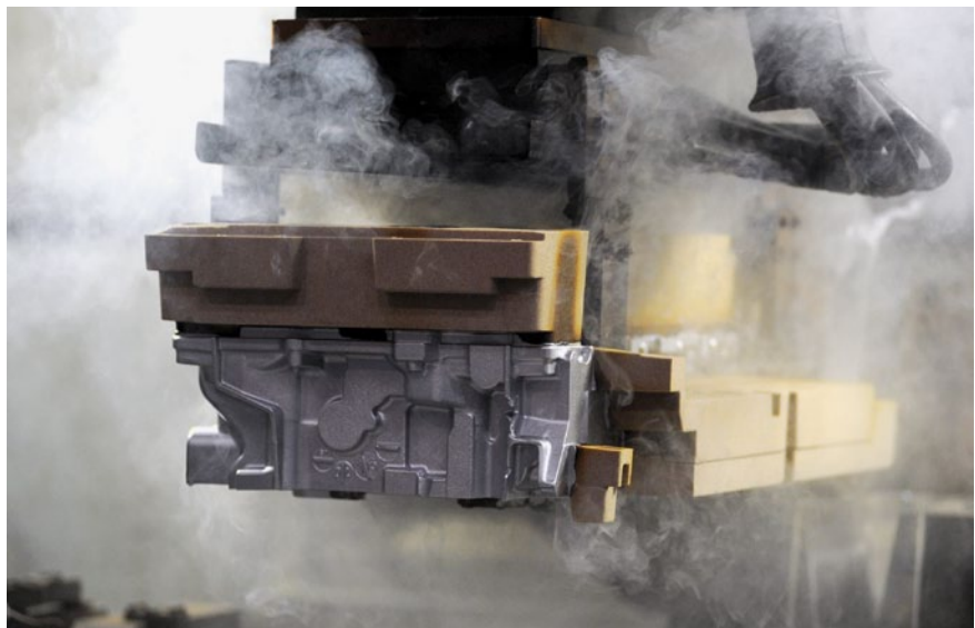
② Core gas developing during casting a cylinder head made with organically bonded cores
