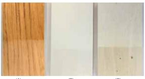
(A) Merbau panel (B) With a white topcoat (C) After 72 hours exposure to the condensation water test
